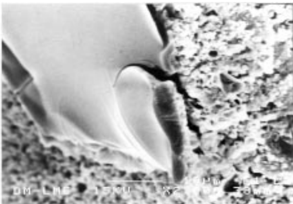
Figure 4 SEM picture of the Biocement F-Glass combination after 2 weeks of aging in 0.5% CaCl 2 solution.
